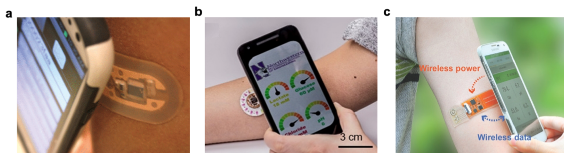
Figure 25. Wireless energy harvesting from the mobile phone. a , A bandage-like RFID sensor patch for the monitoring sweat \text{Na}^+ . Reproduced with permission from ref 473. Copyright 2015 IEEE. b , A soft epidermal microfluidic device integrating an NFC-based wireless monitoring of sweat glucose and lactate. Reproduced with permission from ref 237. Copyright 2019 The American Association for the Advancement of Science. c , An NFC-based wireless sweat sensor system with a stretchable electrode array for the multiplexed monitoring of sweat \text{Na}^+ , \text{K}^+ , pH, and glucose. Reproduced with permission from ref 474. Copyright 2019 Wiley.
